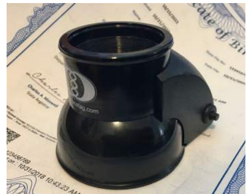
One of the compact, hand-held verifier models for the ValiMark® luminescent materials
